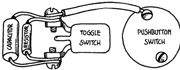
3. Take one wire from the resistor (the small part, usually brown, with the colored bands on it) and attach it to one of the terminals on the toggle switch; attach the other wire to the other terminal of the toggle switch. (Just wrap the wires around the terminal screws, but don't tighten them yet.)
