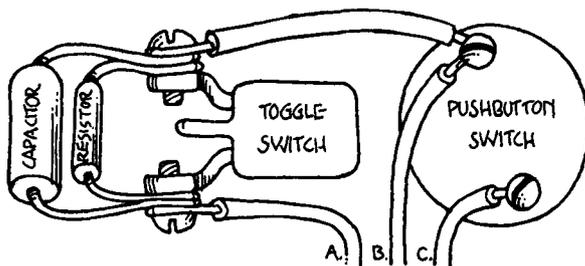
7. Cut a 3- to 5-foot piece of wire (depending on how far you may want to keep the mute box from the phone) and attach one end of it to the terminal of the toggle switch which is *not* connected to the doorbell button (now you can tighten this terminal). Label this wire "A".
